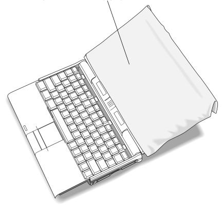
11 Lift the keyboard out of its enclosure and place it on the clean, dry cloth covering the display.
